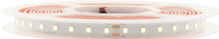
For operation, a supply voltage of min. 23V required. Each segment may be operated with a maximum of 70mA, through parallel connection the currents add up. If the luminous flux listed in the table is not 100% required, the Flexstrip CC can also be supplied with lower currents, which also reduces the connected load. When using appropriate power supplies, a flicker-free amplitude dimming is possible.
