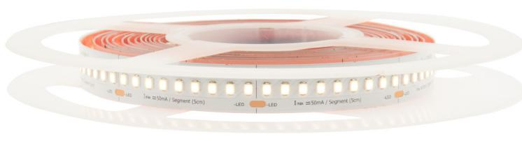
For operation, a supply voltage of min. 23V required. Each segment may be operated with a maximum of 50mA, through parallel connection the currents add up. If the luminous flux listed in the table is not 100% required, the Flexstrip CC can also be supplied with lower currents, which also reduces the connected load. When using appropriate power supplies, a flicker-free amplitude dimming is possible.
