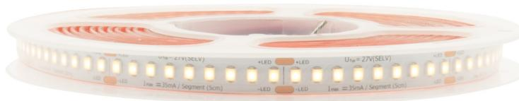
For operation, a supply voltage of min. 23V required. Each segment may be operated with a maximum of 35mA, through parallel connection the currents add up. If the luminous flux listed in the table is not 100% required, the Flexstrip CC can also be supplied with lower currents, which also reduces the connected load. **When using appropriate power supplies, a flicker-free amplitude dimming is possible.**
