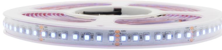
5m reel LED Flexstrip with 50cm long connecting cable at the beginning and end of the strip, with 0.75mm<sup>2</sup> cable cross section. Strip encased in a highly transparent heat shrink pipe with TESA double-sided adhesive tape on the back. Each package includes a 10cm long piece of heat shrink pipe with hot melt adhesive, to seal the end and the beginning of the strip after the assembling.
