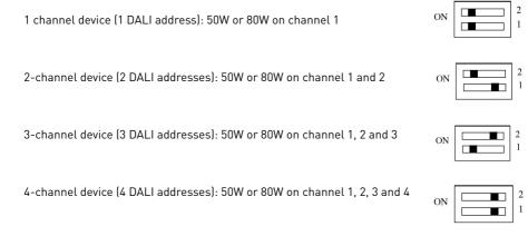
The maximum output power of 50W or 80W is adjusted to the respective set output channels.
